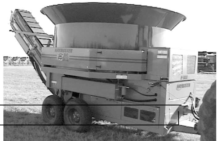
one of three PTO lubrication point, zerk is behind cowling (Ref #12) input shaft bearing lubrication point two of two is in this general area (Ref # 4)
