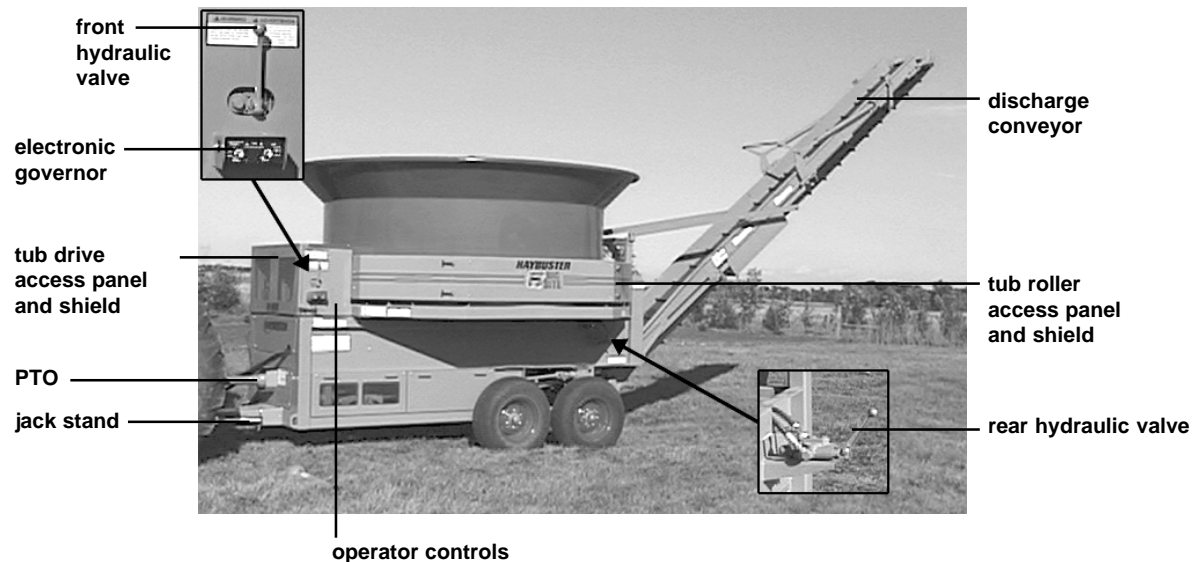
Figure 3.1 side view showing operator station and major system components
