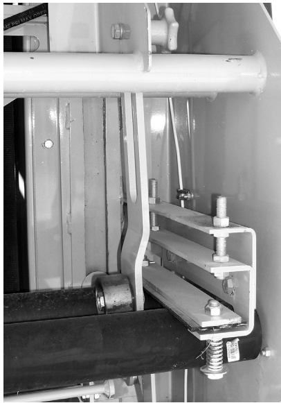
support rollers before the roll of net has been added
