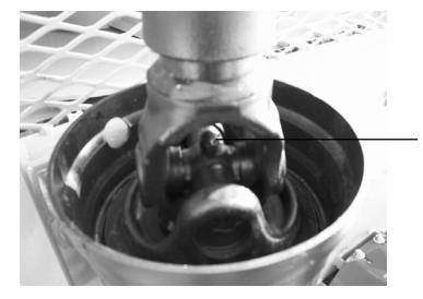
P.T.O. universal joint lubrication zerk
