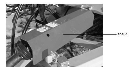
figure 1.2 Orbit motor auger drive sheild
