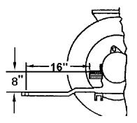
figure 3.6 Safe P.T.O. distance
