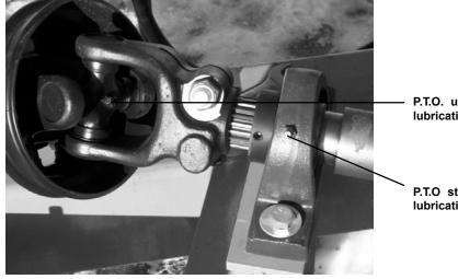
P.T.O. universal joint lubrication zerk
