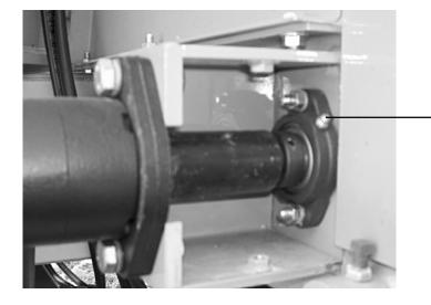
figure 4.8 Extention conveyor bearings lubrication point (1 of 4)
