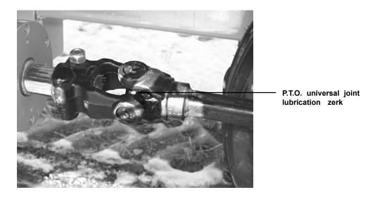
figure 4.6 P.T.O. Universal joint (7 of 7), and automatic clutch
