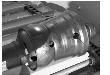
P.T.O. universal joint lubrication zerks
