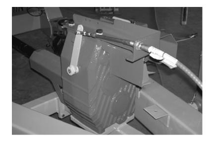
figure 6.8 Handle for two speed gearbox in high position
