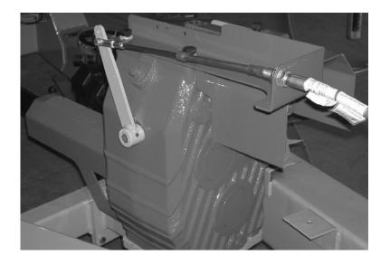
figure 6.6 Handle for two speed gearbox in low position
