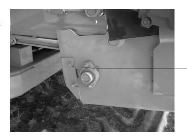
extention conveyor bearings lubrication zerk
