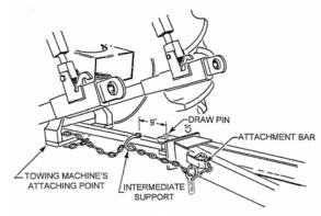
figure 3.7 Safety chain installation
