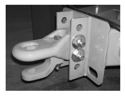
The hitch pin should be of proper diameter to prevent movement and length to extend through all components of the hitch. The pin should be secured with a hairpin clip or suitable device to prevent the loss of the pin.
