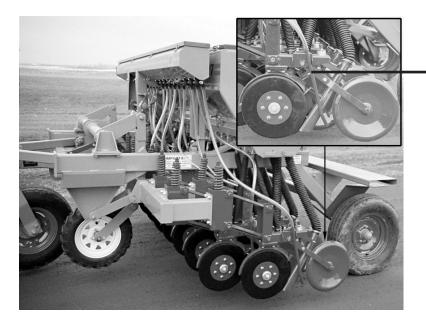
drop tube with seed tube connected
