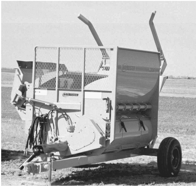
Rack and deflector in transport position
