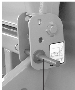
loader transport pin in storage position
