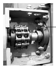
conveyor bearings lubrication zerk
