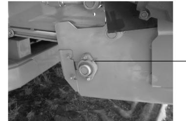
extention conveyor bearings lubrication zerk
