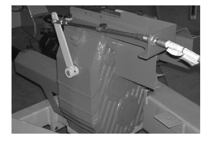
figure 3.8 Handle for two speed gearbox in high position
