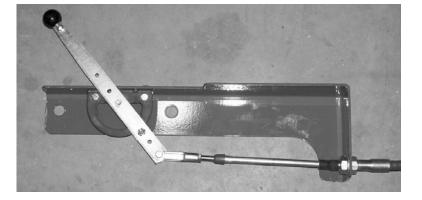
figure 3.9 Two speed gearbox in high position
