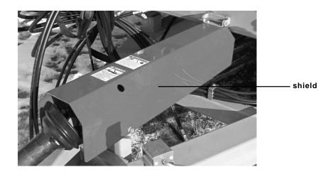
figure 1.2 Orbit motor auger drive shield
