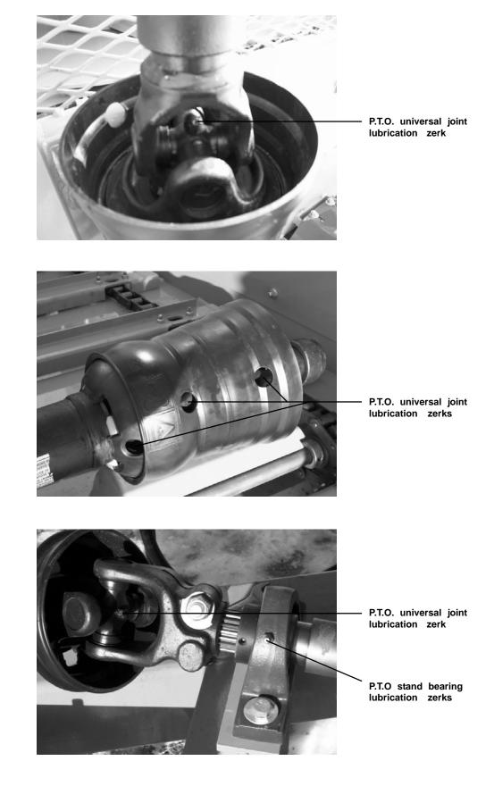
figure 4.2 P.T.O. Universal joint (2, 3, & 4 of 8)
