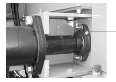
conveyor bearings lubrication zerk
