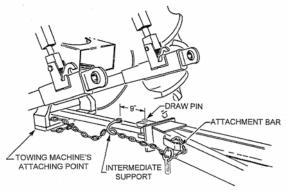
figure 3.7 Safety chain installation
