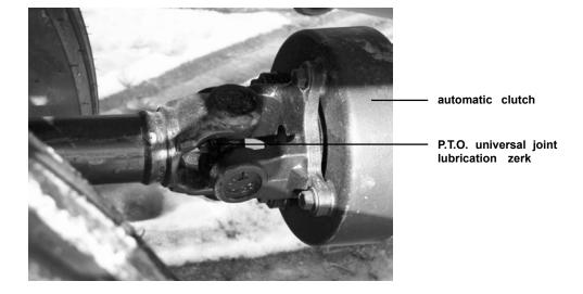
figure 4.5 P.T.O. Universal joint (6 of 7)
