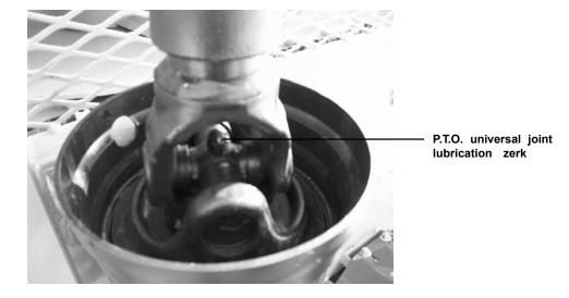
figure 4.2 P.T.O. Universal joint (2 & 3 of 7)
