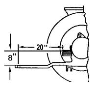
figure 3.6 Safe P.T.O. distance
