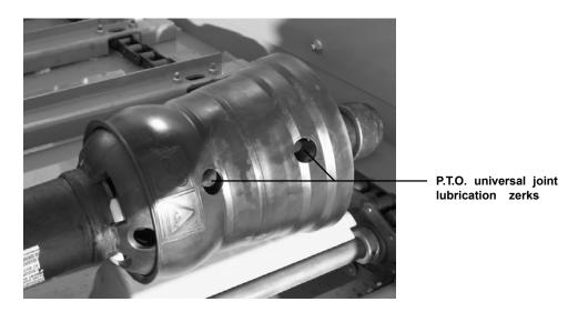
figure 4.3 P.T.O. Universal joint (4 of 7), and P.T.O stand bearing (1 of 1)
