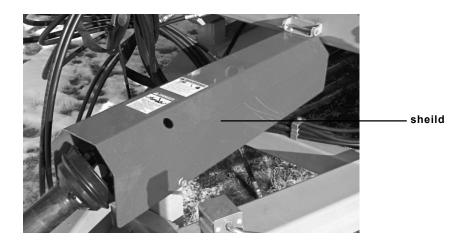
figure 1.2 Orbit motor auger drive sheild
