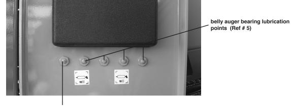
front rotor bearing lubrication points 2 of 2 (Ref # 3)
