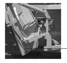
discharge conveyor bearing lube points -one on each side of machine (Ref #7)
