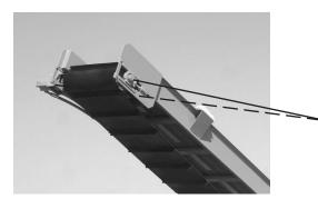
discharge conveyor bearing lube points (Ref #7)
