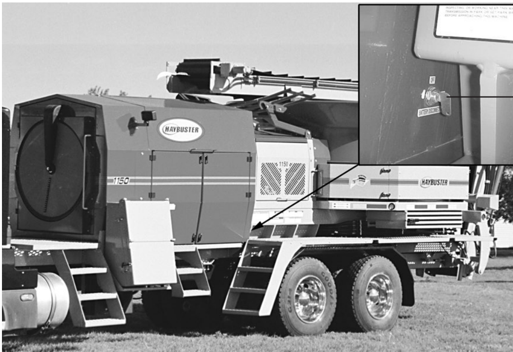
battery disconnect switch
