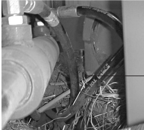
figure 5.2 rotor bearing vent and sight glass
