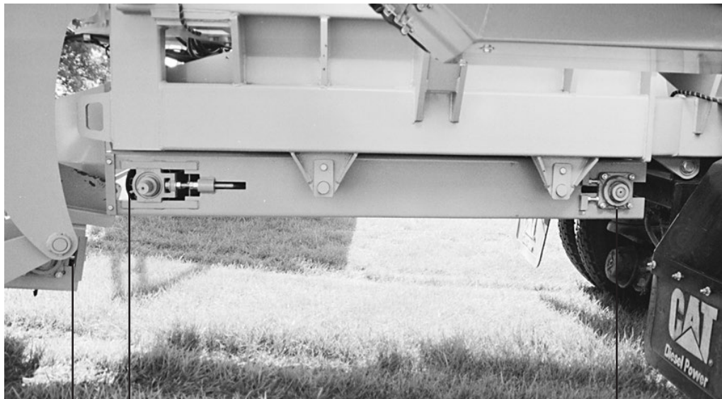
figure 5.5 belly conveyor roller & discharge conveyor roller lubrication points
